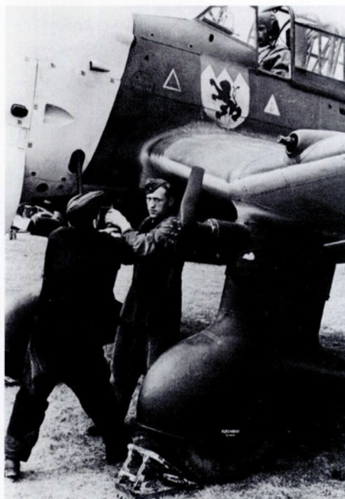
Ground crew preparing to start the engine of a Ju 87 B-1 of Stab II./St.G 77 in the Balkans. The yellow campaign marking on the cowling has evidently just been applied as there is no sign of any exhaust staining. Note the engine starting handle and the propellers for the wind driven sirens.
