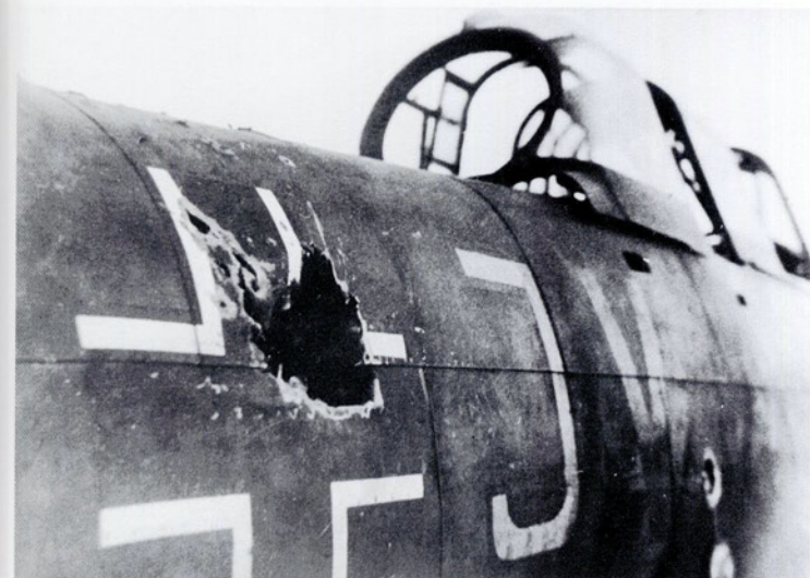
Two views of Flak damage sustained by a Ju 87 B, W.Nr. 0236, during the campaign in Poland in September 1939 and which made a forced landing at Grieslinen in East Prussia, losing its undercarriage in the process. The photograph above shows the starboard side where the shell entered the fuselage and exploded, blowing out a large part of the aircraft's port rear fuselage. The port fuselage has separated along the joint where the upper and lower fuselage shells are joined in the manufacturing process - an unusual method of construction. This particular machine was coded L1+JV and belonged to IV. (Stuka)/Lehrgeschwader 1.
