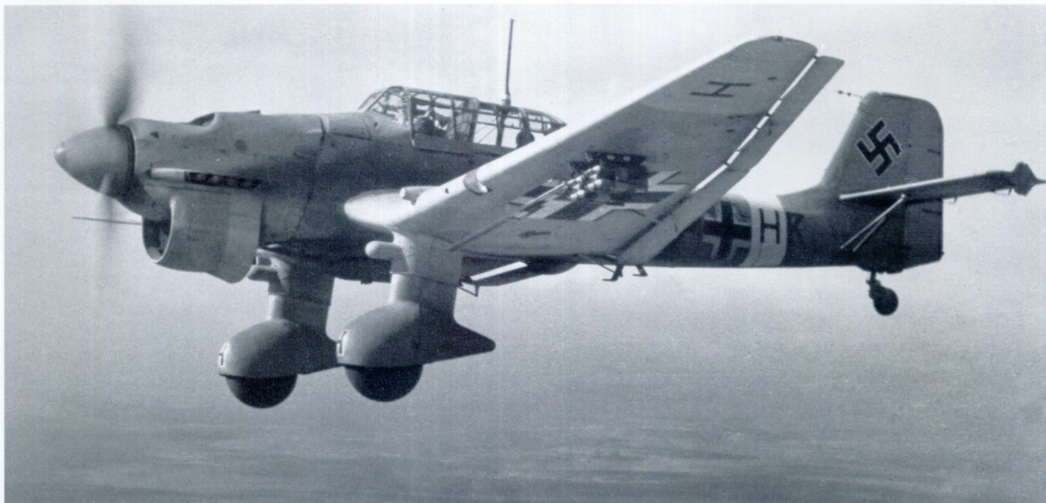
Some machines, particularly those of St.G 3, were recamouflaged in an overall tan finish. The full operational code on this Ju 87 R-2 of 2./St.G 3 shown flying over North Africa, was S1+HK. Note the SD 10 anti-personnel bombs carried in two bundles of five under each wing.
