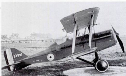
A production example of the British S.E.5a fighter of 1917-18, s/n B'4897, with a strengthened undercarriage. This type of aircraft was used by the fledgling RAF to conduct dive-bombing trials and a machine flown by 2nd Lt William Brown of No.84 Squadron carried out the first known combat dive-bombing mission.
