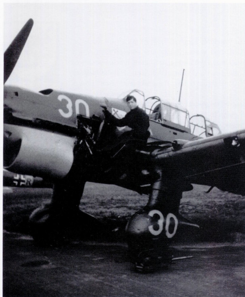
A groundcrew mechanic has removed the rear side access panel to the Jumo 211 engine of '30' in order to carry out some routine maintenance. The Ju 87 B-1s were fitted with Jumo 211 A fitted with Junkers Ju HPC, 3.4 metre diameter propellers while the Ju 87 B-2 was fitted with Jumo 211 Ds and VS 5, 3.4 metre diameter propellers.
