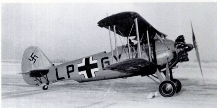
The Heinkel He 50 biplane was used in small numbers by JG 132 shortly after its formation in order to experiment with dive-bombing. Originating from a Japanese specification for a two-seat dive-bomber, it was a particularly strong aircraft able to withstand high diving speeds. It played a key role in Germany's pre-war dive-bombing development. Trials were conducted using cement 'bombs' at Rechlin and Warnemünde. This example, LP+GY, was attached to a training unit based in Czechoslovakia in 1939-40. The aircraft was finished in RLM 02, features a pre-war positioned Hakenkreuz and coloured wheel spats, possibly in black or red.
