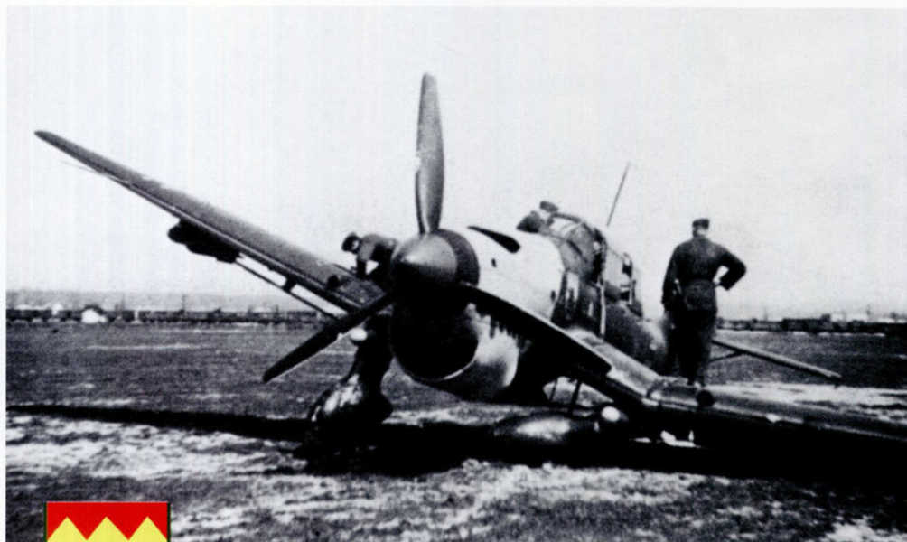
Ju 87 B-1 of Stab II./St.G 77 in the Balkans. This aircraft, flown by the Kommandeur, has suffered a collapsed port undercarriage.
