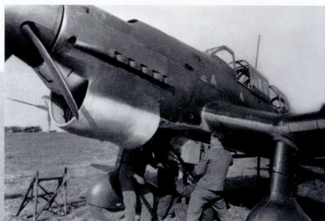
A Ju 87 B of an unidentified unit is being prepared to be used as an improvised 'transporter'. Here, ground crew make ready the bomb rack to receive a large wooden heavily padlocked chest in place of the usual bomb load, in order to transport equipment – probably essential tools – to the next forward airfield. Note the 'L' denoting the individual aircraft code painted on the lower cowling just aft of the spinner and the SD 50 fragmentation bomb fitted with whistles lying on the grass just in front of the port undercarriage.
