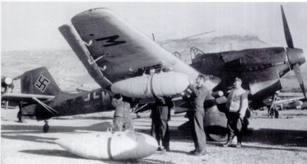
Ju 87 R-2s, of I./St.G 2 carrying the unit code T6, being fitted with underwing tanks and refuelled somewhere in the Mediterranean theatre. This Gruppe operated from various bases in Italy, Greece and North Africa throughout 1941; though there is an absence of the usual white theatre band on most of these aircraft, the third aircraft in the line-up does have one painted around the fuselage Balkenkreuz. This suggests that they were photographed early in their deployment, possibly at Trapani. Note the individual aircraft letter M under the wingtip.
