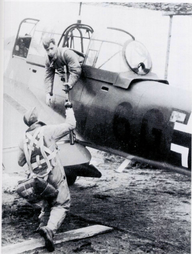
The pilot of a Ju 87 B-1 of III./St.G 51 passing the wireless operator/gunner his 7.9 mm MG 15. When the Ju 87s encountered determined aerial opposition, this weapon proved inadequate. Note the original Gruppe badge which comprised a silver mailed fist on a yellow shield.
